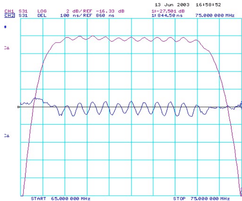
Fig-2 Group Delay and Ripple, Horizontal:1MHz/Div Vertical: 2 dB/Div Vertical: 100nS/Div
